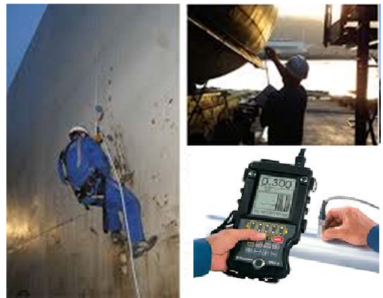
Fig. 2 Action of thickness measurement and equipment
