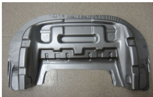
Fig. 12 Drawing process of seat cushion panel
