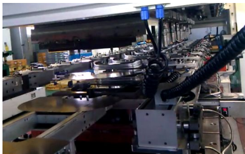
Fig. 19 Press line of semi-progressive die and transfer die
