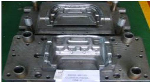
Fig. 17 Drawing process of developed transfer die
