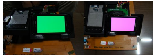
Fig. 13 Photos of the display function test of the separated LCD modules
