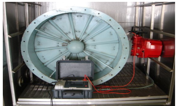
Fig. 9 Environmental test apparatus for vane damper
