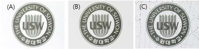
Figure 1. Photographs of PEDOT/PSS coated on PET film when binder was PVA (A), PVP (B), and PSS (C).
