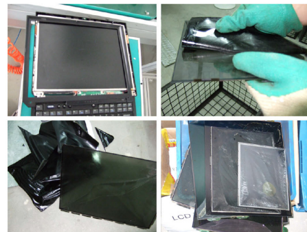
Figure 2. The changes of ITO glass appearance through thermal-shocked treatment at the temperature 230 °C such as the bugling and delamination of surface polarizing film[8].
