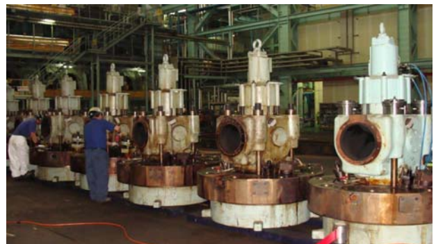
Figure 3: Exhaust valve of the test engine
