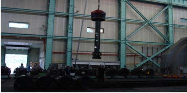
Figure 4: Piston of the test engine
