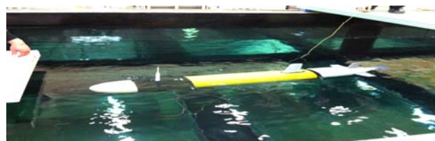
Figure 7: Measurement of the drag force of AUV
