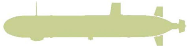
Figure 5: projected area of the side of AUV
