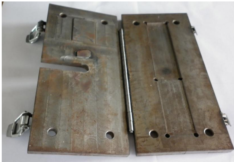
Figure 3. a jig for setting up the experimental specimen.
