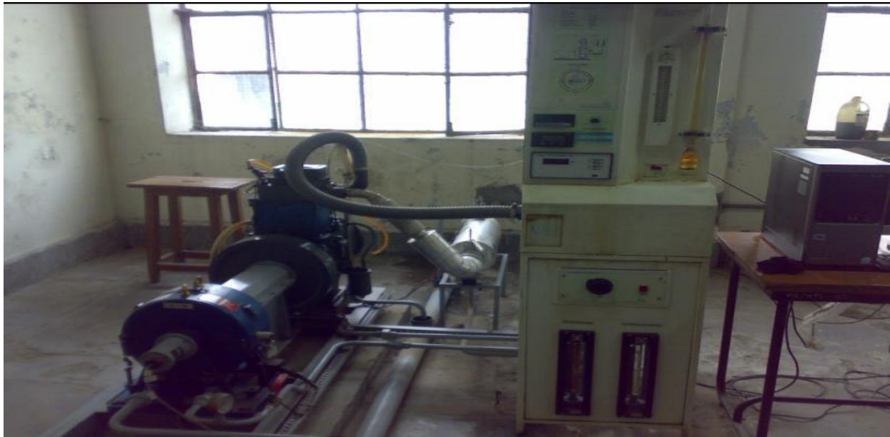
Photo 1. Variable Compression Ratio Engine with Loading Unit & Data Acquisition unit attached
