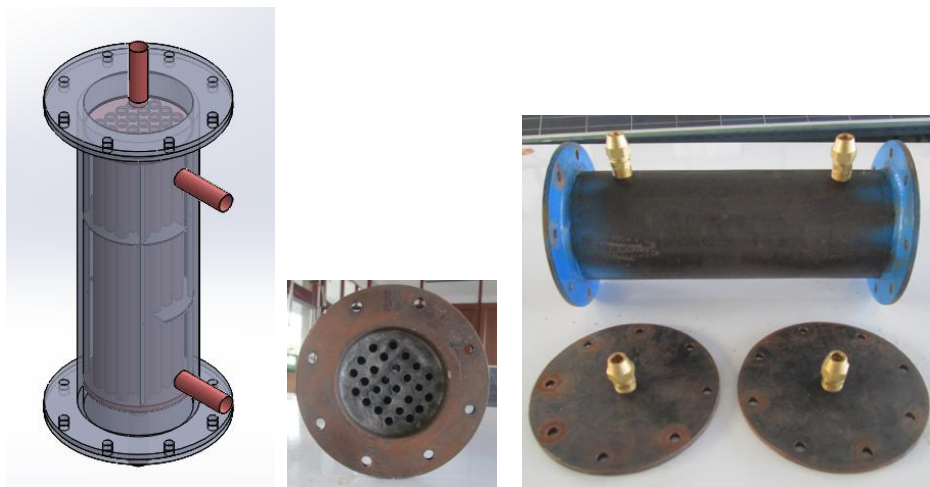
Figure 8. Shell and Tube Heat Exchanger for compered calculating with Fig 7.
