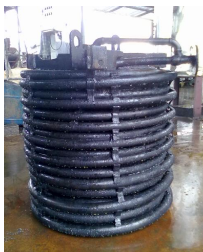
Figure 5. Spiral coil in Heat Exchanger. [7]
