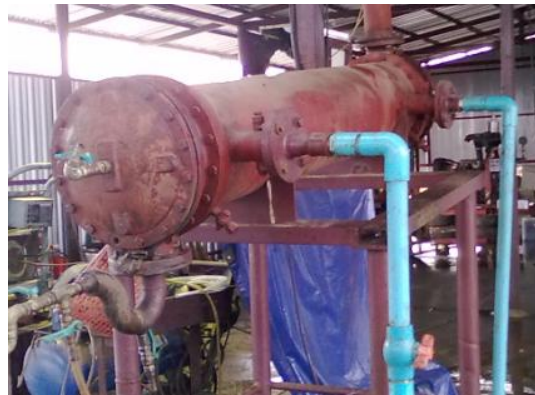
Figure 7. Shell and Tube Heat Exchanger. [7]
