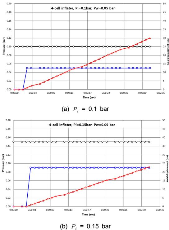
Fig. 8. Water pressure & axial displacement with time for 4-cell inflater
