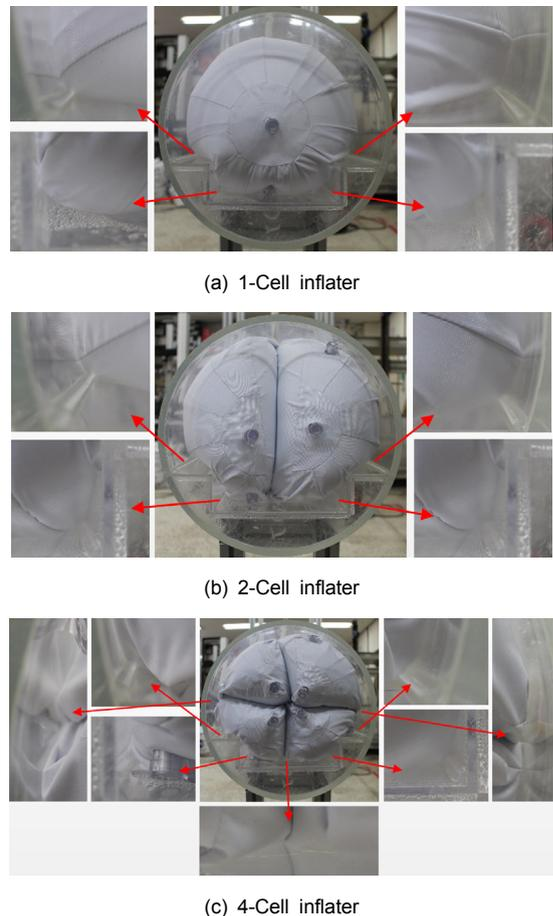
Fig. 5. Types of multi-cell inflaters
