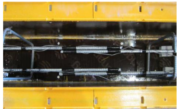
Fig. 4 Lap splices in concrete beam
