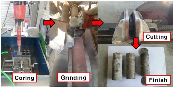
Fig. 3 Manufacturing process of testing specimen
