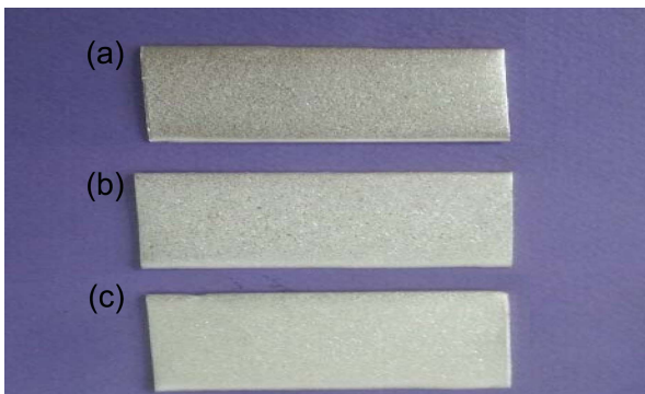
Fig. 7. Continuous and uniform thickness thin tape well shaped. (carrier speeds, a: 42 cm/min., b: 60 cm/min., c: 75 cm/min.).
