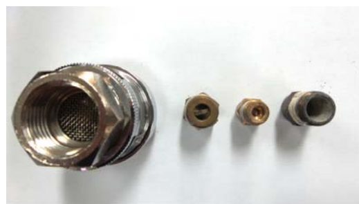
(e) 3-prong, (f) circular(3 mm), (g) circular(1.5 mm) (h) ellipse (B) Rear view
