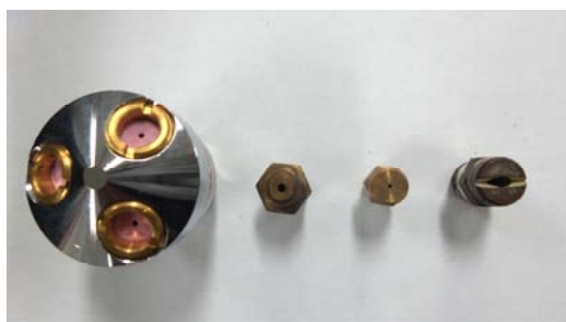
(a) 3-prong, (b) circular(3 mm), (c) circular(1.5 mm) (d) ellipse (A) Front view
