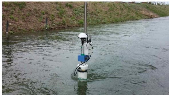
Fig. 5. ADCP and RTK-GPS
