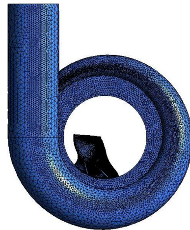
Fig. 5 The surface grid of the vaneless diffuser, volute domain, and one passage impeller
