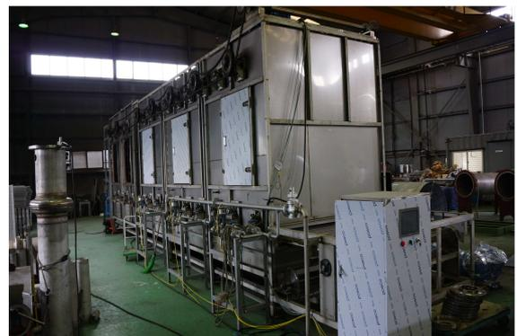
Fig. 9 Experimental apparatus of sterilizer for this research
