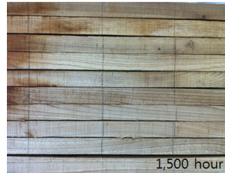
Fig. 3. Visual Identification for Wood Specimen in Weathering time.
