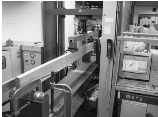
Fig. 1. Set up for structural lumber bending test (Hwang et al. 2011).
