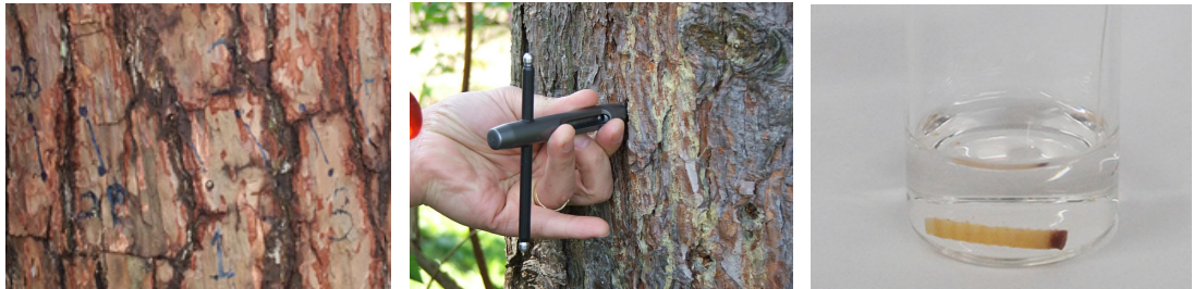
Fig. 1. Left: sampling points, Middle: collecting samples using Trephor ( \varnothing 1.9 mm) (middle), Right: mini core.
