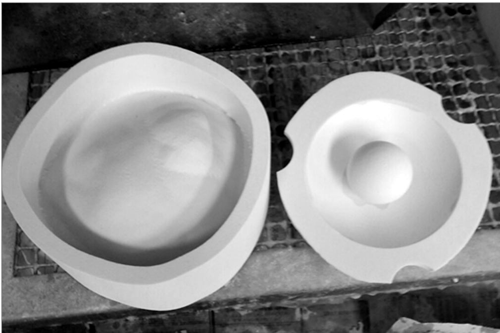
Fig 5. Molding box for customized bolus.
