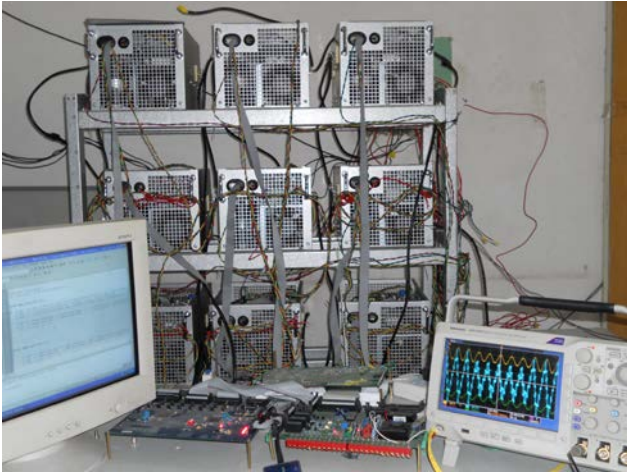
Fig. 11. Photo of the single-phase MMC-based inverter.
