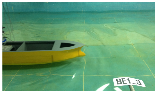
Fig. 2. Wave pattern for VLCC model (even keel, \lambda/L = 0.7 , F_n 0.091, ballast condition).
