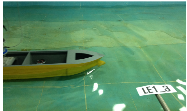
Fig. 1. Wave pattern for VLCC model (even keel, \lambda/L = 0.7 , F_n 0.091, full load condition).
