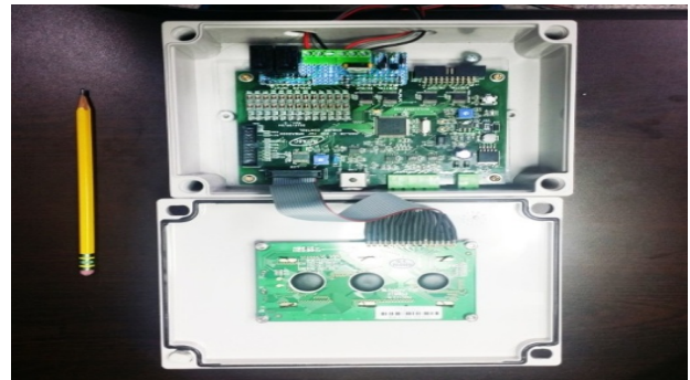
Figure 17: Controller on an embedded system
