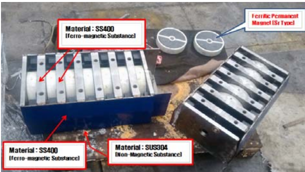
Figure 9: Image to show the relationship between the individual components and the relevant materials used for the permanent magnet body
