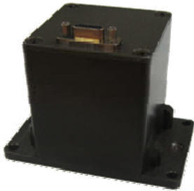
Figure 1: AHRS based MEMS for small high speed UUV.
