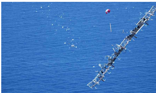
Fig. 1. Failure by divergent pitch mode
