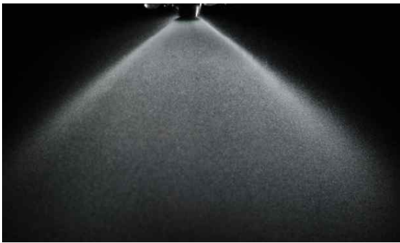
Fig. 14. Scattering image of spray at 0.4 mm of opening distance
