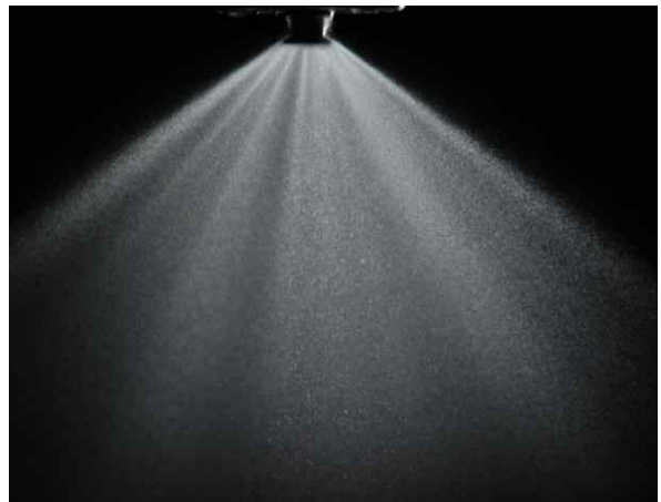
Fig. 12. Scattering image of spray at 0.2 mm of opening distance
