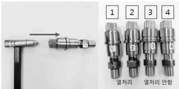
Fig. 12. Input shaft heat-treat check test.
