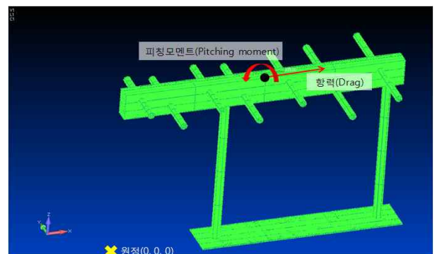
Fig. 9 Load applied on the finite element model
