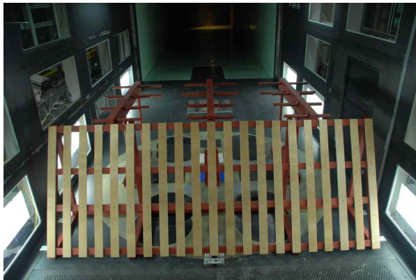
Fig. 4 Deflector at front of localizer in the test section
