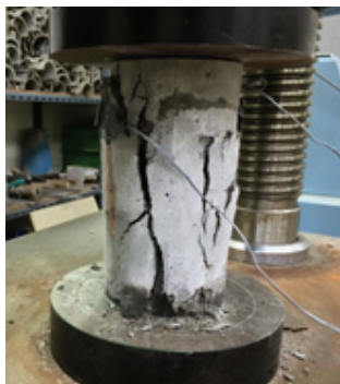
Fig. 2 Compressive stress test
