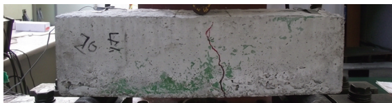
Fig. 5 Failure Mode of Concrete Beam Mixed with 4% of SSPCM
