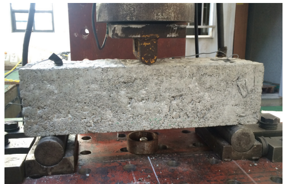
Fig. 4 Flexural-Shear Stress Test Set Up
