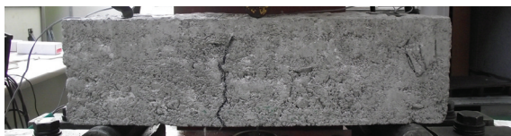
Fig. 6 Failure Mode of Concrete Beam Mixed with 6% of SSPCM
