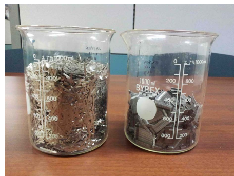
Fig. 2. Apparent solid volume : amorphous steel fiber vs. hookend steel fiber.
