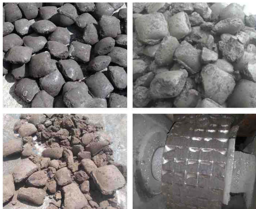
Fig. 4. Formability evaluation of CCBI through visual inspection. Formability is divided into four categories with the highest formability having an index of 4 with non-formability corresponding to an index of 1.
