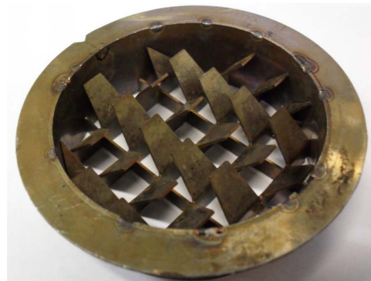
Fig 4. Spray droplet breaker plate
