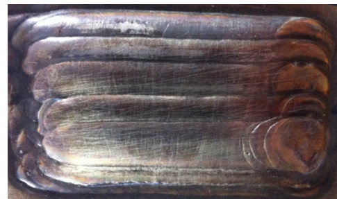
Fig. 5 Bead appearance of ER2594 welded with 98%Ar-2%N 2
