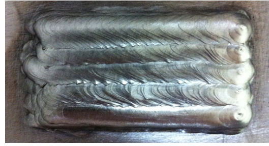
Fig. 3 Bead appearance of ER308L welded with 98%Ar-2%N 2
