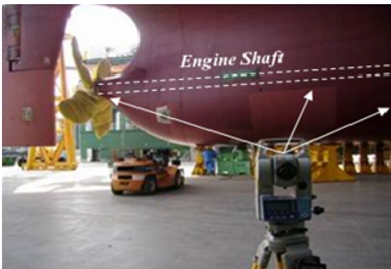
Fig. 1 Centering at the erection stage
