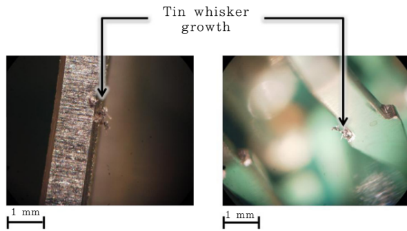
Fig. 11 Tin whisker growth on tin-finished connector pin in automotive ECU 15)
