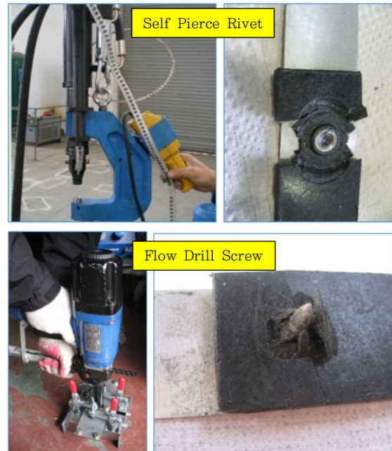
Fig. 14 Results for each mechanical fastening processes (SPR and FDS) to make aluminum and plastic joining
