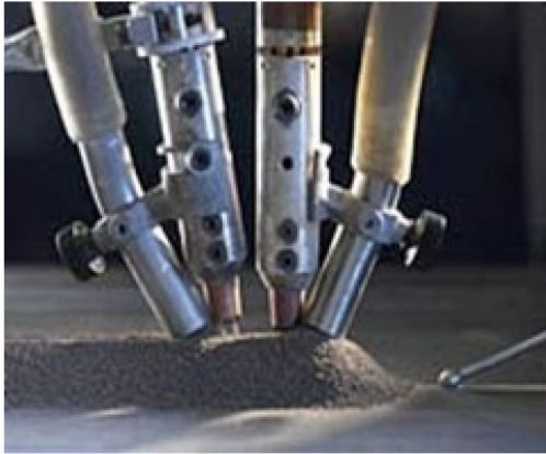
Fig. 4 Tandem SAW method 6)
