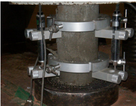
Fig. 1 Test setup for modulus of elasticity
