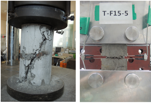
Fig. 3 (Left) Compressive strength test and (Right) Direct Tensile strength test of UHPFRC
