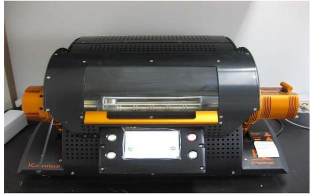
Fig. 6. Automatic fusion equipment (K2 Prime).
