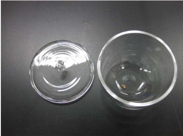
Fig. 3. Air filter after 450 °C, 15 hr ashing.
