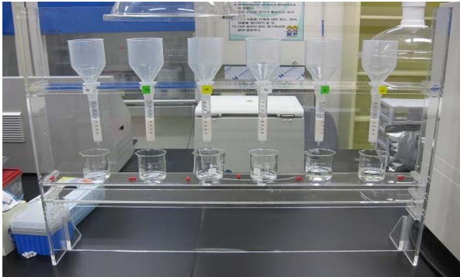
Fig. 8. UTEVA resin, column and column wrack.
