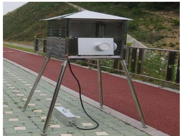
Fig. 2. Automatic air sampler used for collection of uranium particle.
