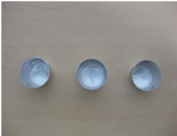
Fig. 5. Folded air filter and LiBO<sub>2</sub> in Pt crucible.
