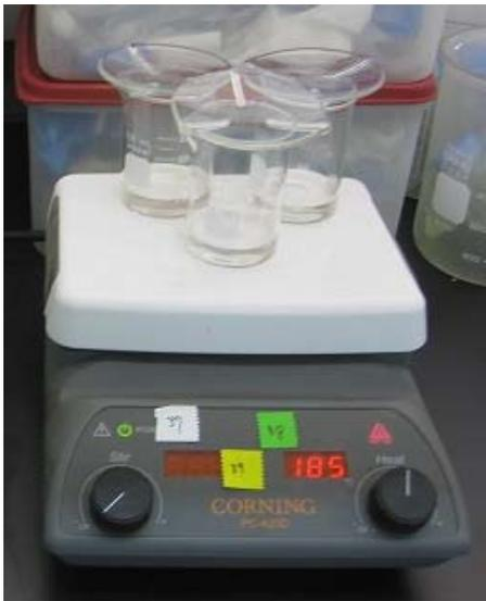
Fig. 4. A digital hot plate and stirrer.
