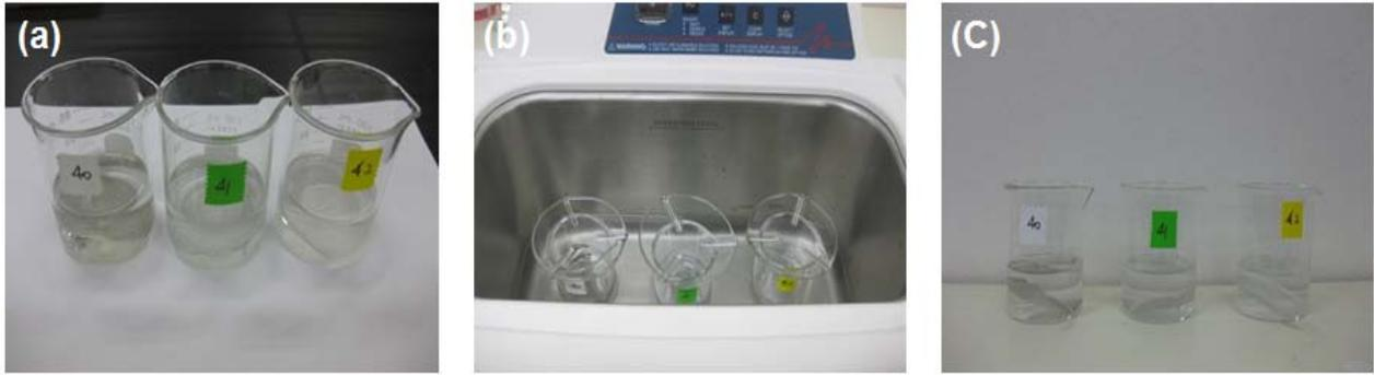
Fig. 7. The process of ultrasonic cleaning.
