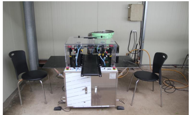
Fig. 1. Grafting robot (GR-600CS) used for experiment.
