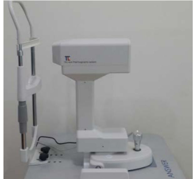
Fig. 4. Photograph of the thermal camera(Cox CX series).
