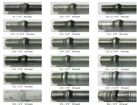
Fig. 5 Manufactured fitting pipe by press forming process
