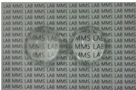
Fig. 9 Comparison of aspheric lens before and after MR polishing
