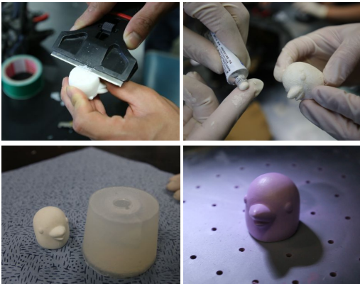
Fig. 3 Photographs of practice; post-processing, sending, RTV and painting.
