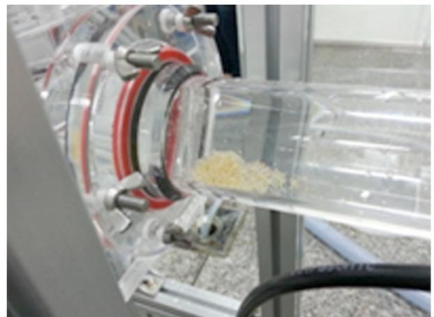
**Fig. 9.** Sand particles deposited at the mouth of pipe B
